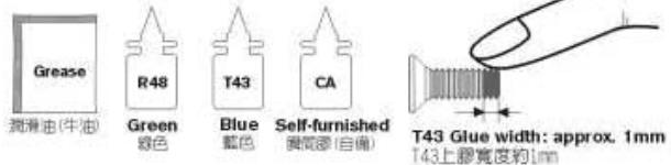
R48 metal tubular adhesive (eg. Bearings). T43 thread lock, apply a small amount on screws or metal parts and wipe surplus off.
